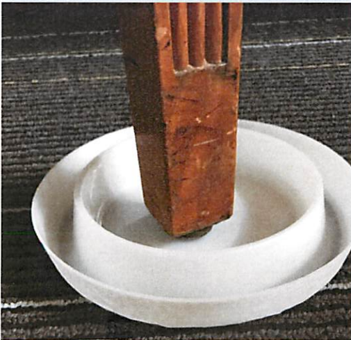
ClimbUp™ monitoring device placed under leg of bed to capture bed bugs
